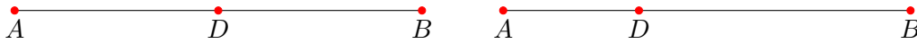
FIGURE 4. The new node on an edge AB . (left): A \neq Q_i and B \neq Q_i (midpoint); (right): A = Q_i ( |AB| = \kappa_{Q_i}|AB| , \kappa_{Q_i} < 0.5 ).
